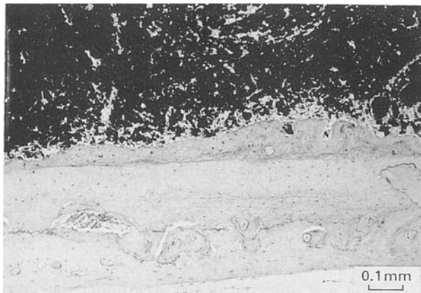
Figure 6 Rat skull (os parietale) 10 weeks after implantation of \text{TiO}_2 powder(black). The \text{TiO}_2 is in close contact with the new bone formed.
